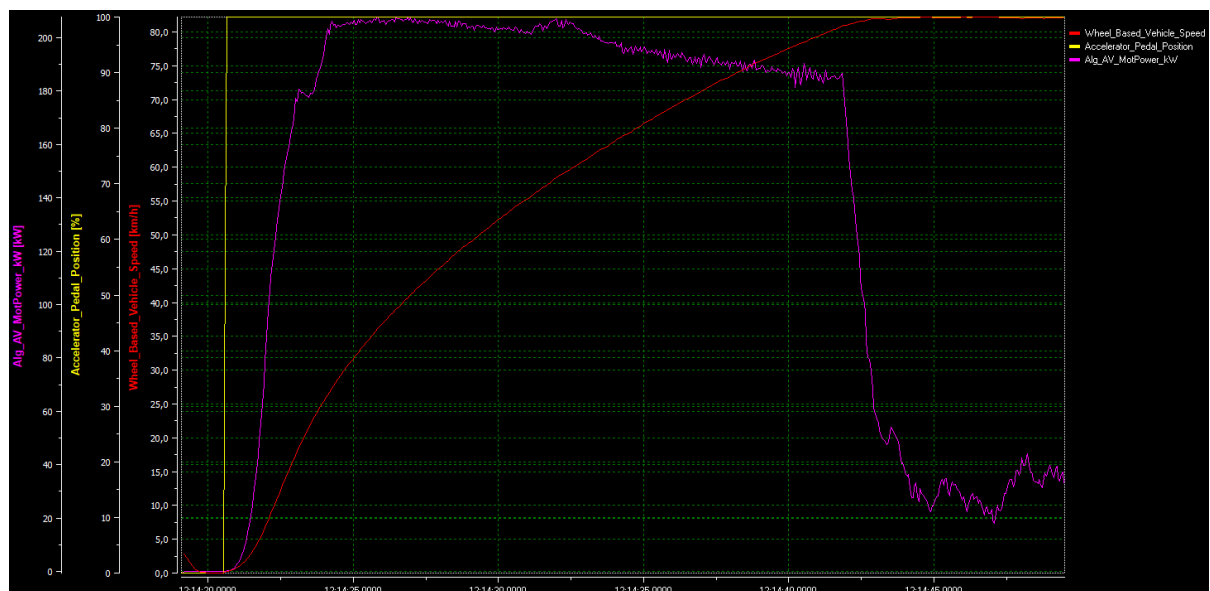
Figure 13. Speed and motor power during full acceleration test
