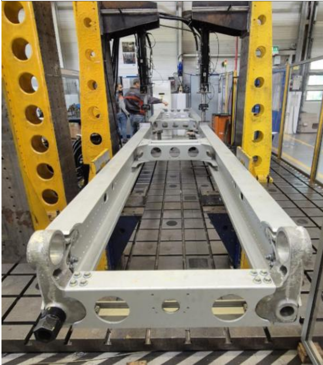
Torsional&Bending Stiffness Test
