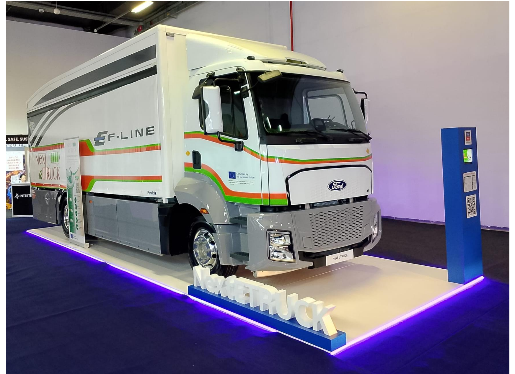
Next e-TRUCK Vehicle 4x2, 16t New BEV Platform
