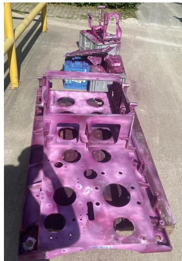
After penetrant spray application
