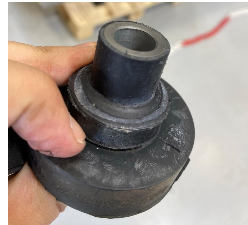
Acceptable wear in mounts (better than rigid e-truck)
