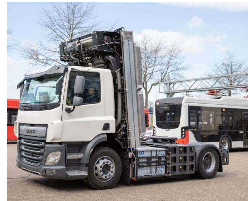
VDL Prototype Truck 44t0 2x FCM50 (A-Sample), 40kg/350bar H2 Tank System, 210kWh Battery
